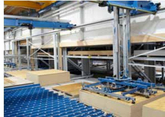
4-axis handling system for panels up to 6 m long
